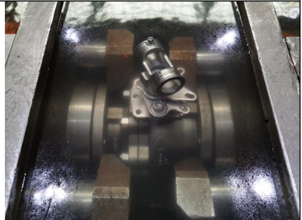
Gas Leak Shell Test
