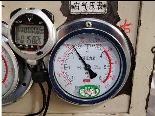
Gas Leak Shell Test
