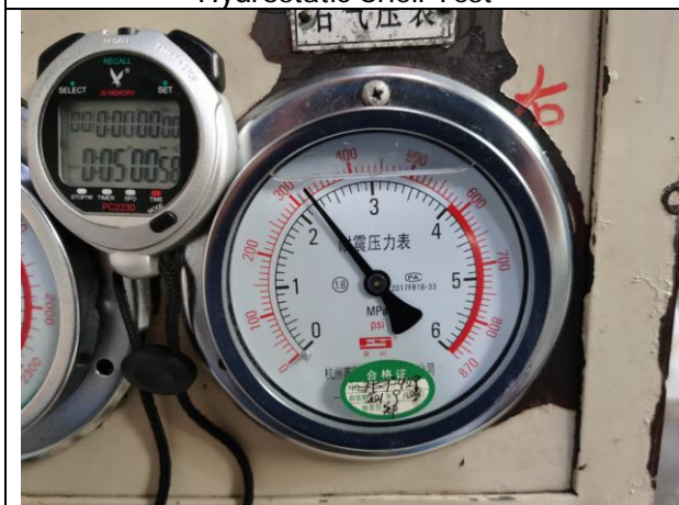
Hydrostatic Seat Test
