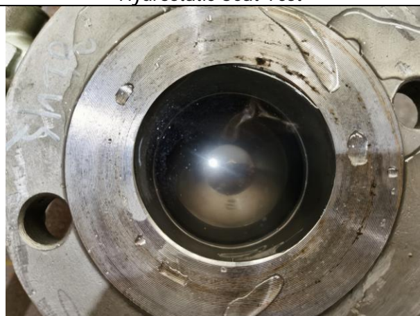
Hydrostatic Seat Test
