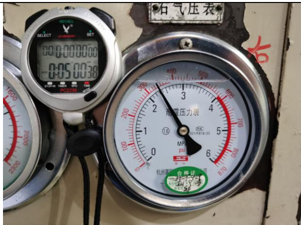
Gas Leak Seat Test
