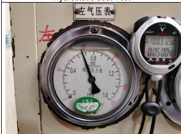
Hydrostatic Seat Test
