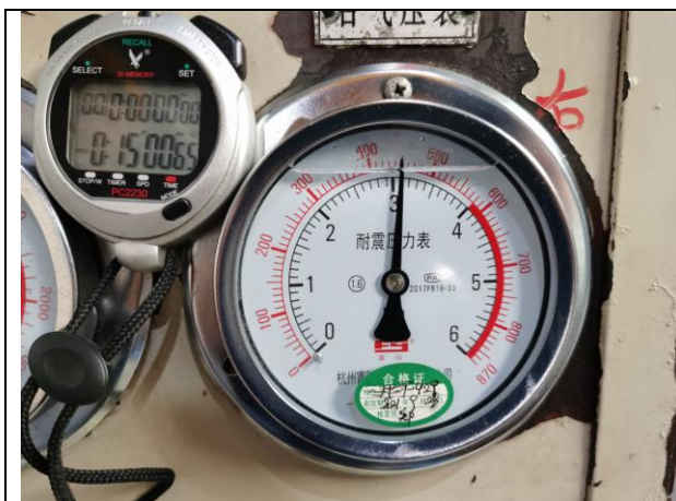
Hydrostatic Shell Test
