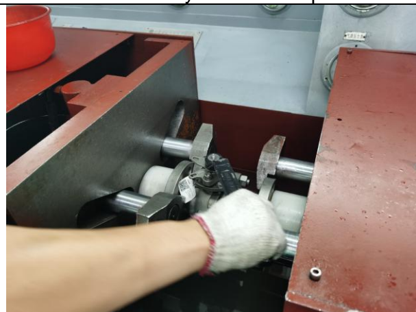
Functional Test - Cycled Close-Open-Close
