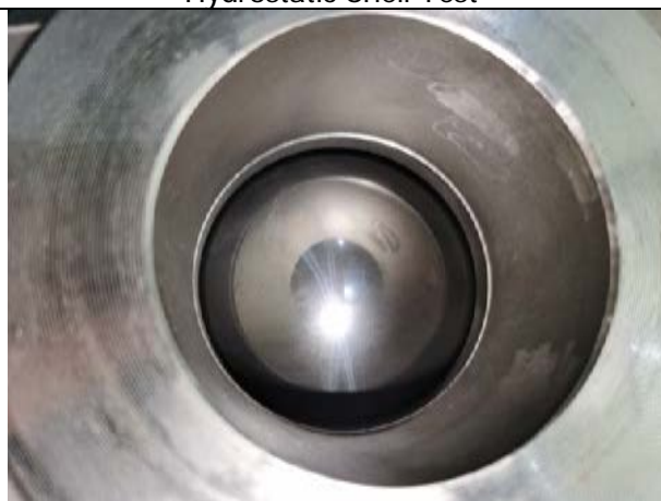
Hydrostatic Seat Test
