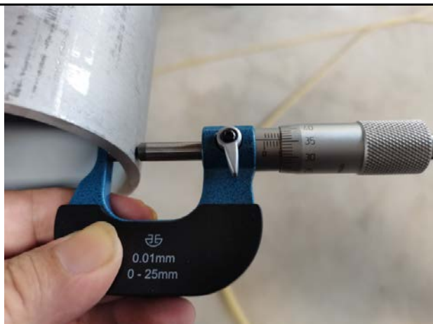
Pipes thickness check
