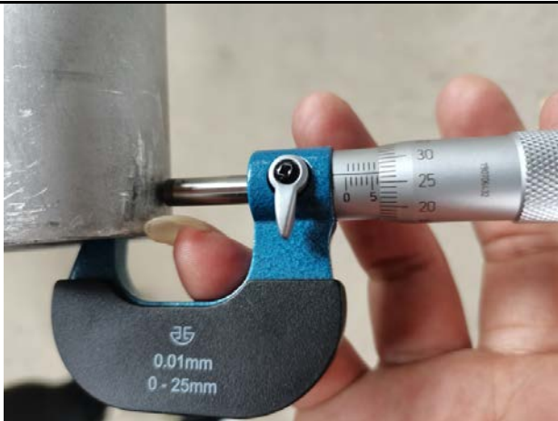
Pipes thickness check
