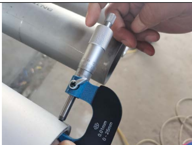
Pipes thickness check
