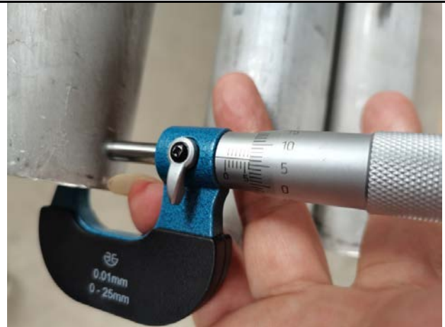
Pipes thickness check
