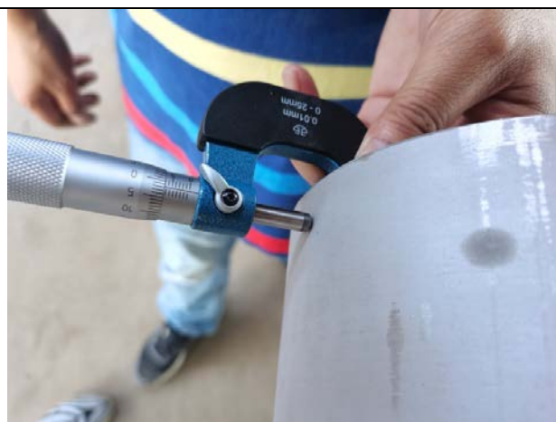
Pipes thickness check
