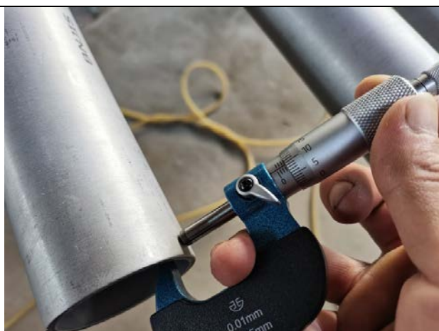
Pipes thickness check
