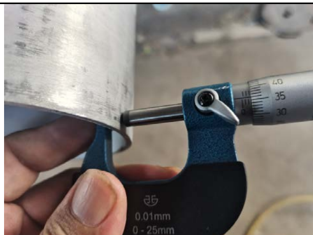
Pipes thickness check
