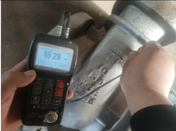
Z10"150LB WT acc. to API600 14.2 mm
