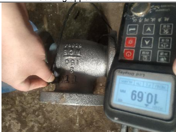
J2"150LB WT acc. to API600 8.6 mm
