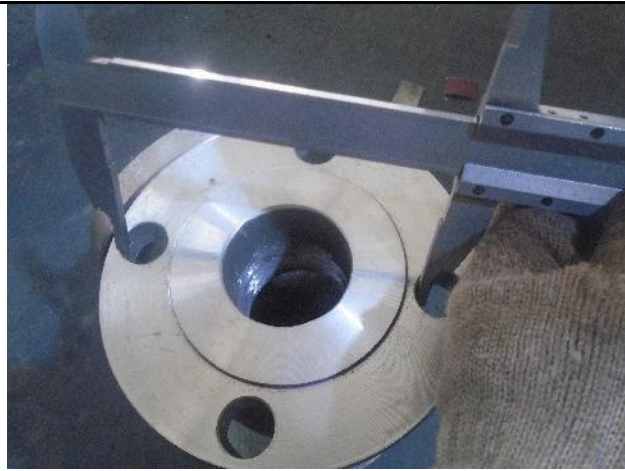
Bolts hole center distance
