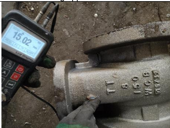
Z8"150LB WT acc. to API600 12.7 mm
