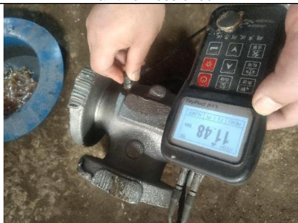
Wall thickness check
