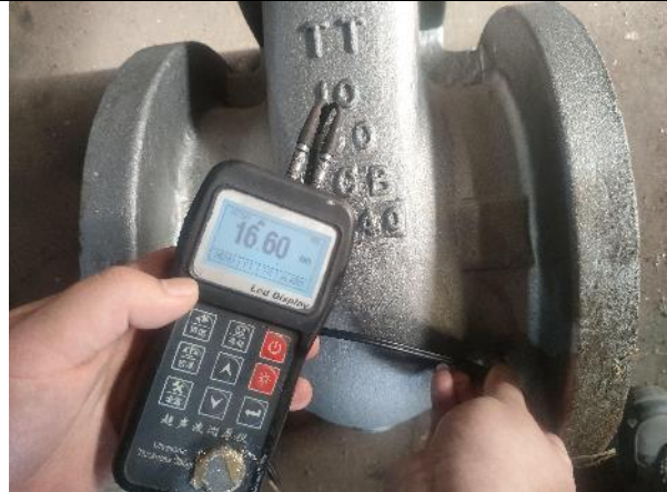
Wall thickness check
