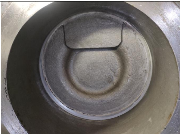
Hydraulic seat sealing test
