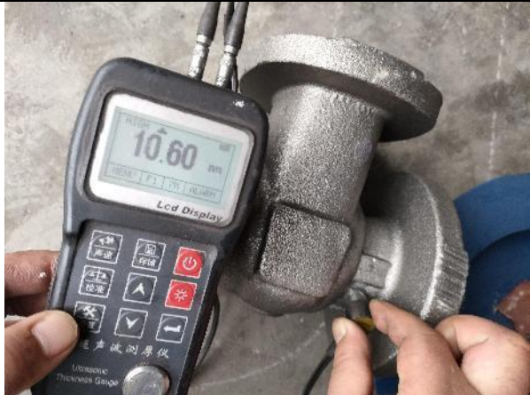
Wall thickness check
