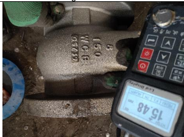
Wall thickness check
