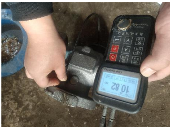
Wall thickness check
