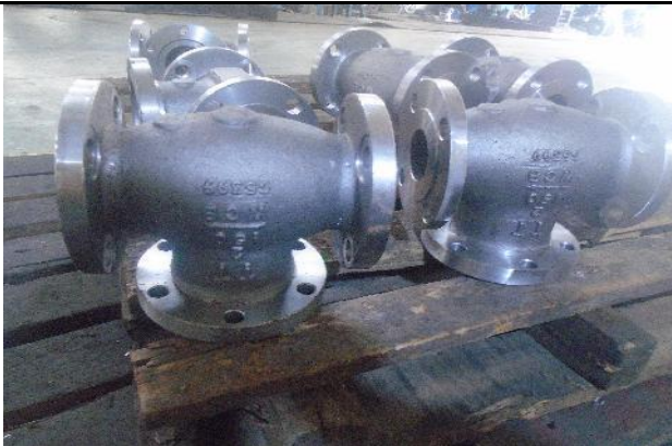
Machining surface check
