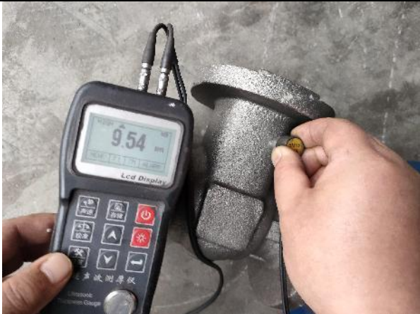
Wall thickness check
