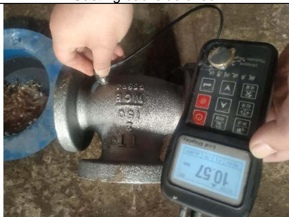
Wall thickness check
