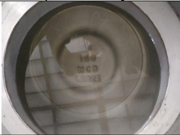
Pneumatic seat sealing test
