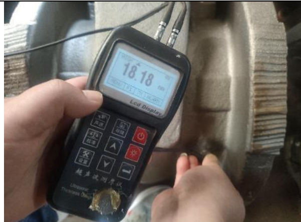
Wall thickness check
