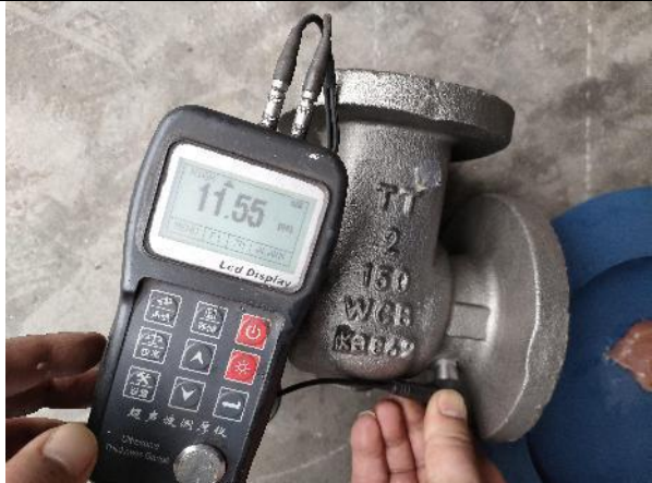
Wall thickness check
