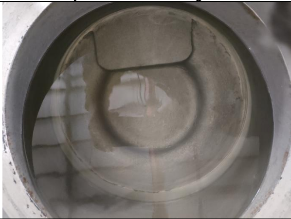
Pneumatic seat sealing test
