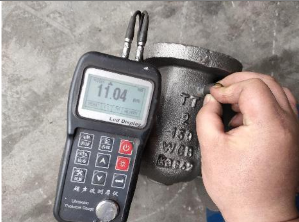
Z2"150LB WT acc. to API600 8.6 mm
