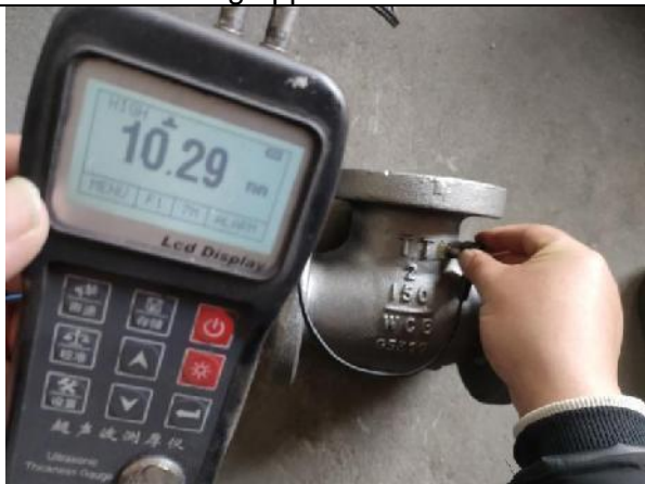
J2"150LB WT acc. to API600 8.6 mm
