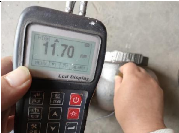
Wall thickness check
