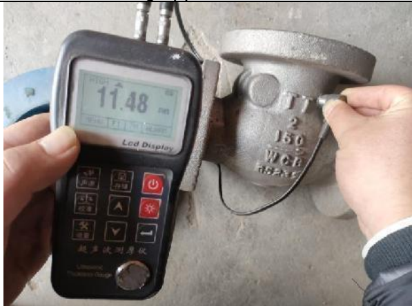
H2"150LB WT acc. to API600 8.6 mm
