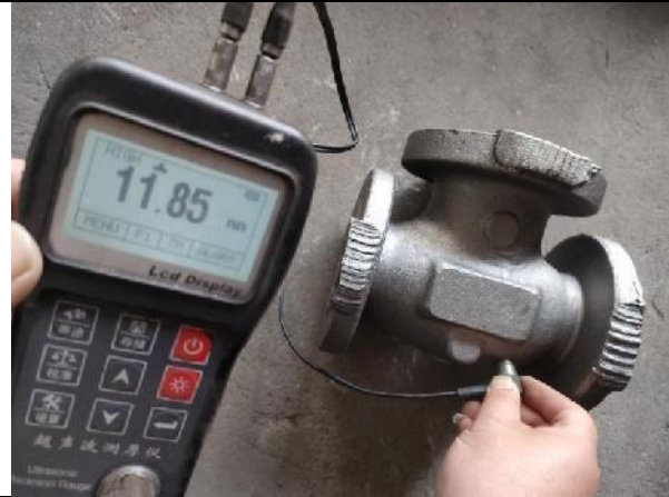
Wall thickness check
