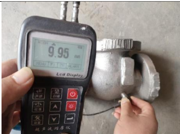
Wall thickness check
