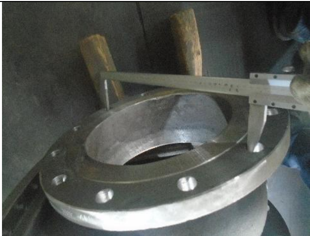
Bolts hole center distance
