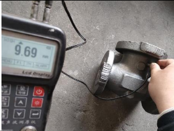
Wall thickness check
