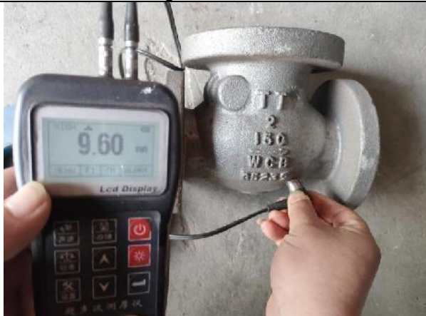
Wall thickness check
