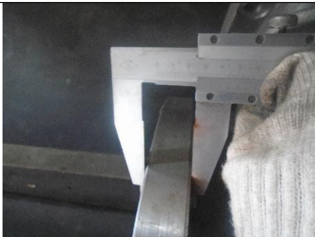
Flange thickness check
