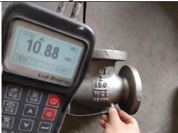
Wall thickness check
